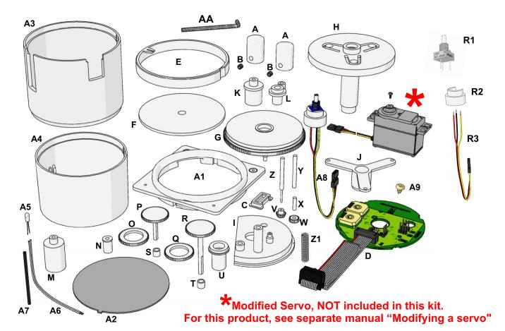
**Construction kit "Heading Indicator"** Your kit contains all the necessary components (except for a servomotor) for building a "Heading Indicator".
