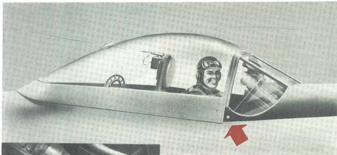
CANOPY CRANK AND EMERGENCY RELEASE INSIDE
