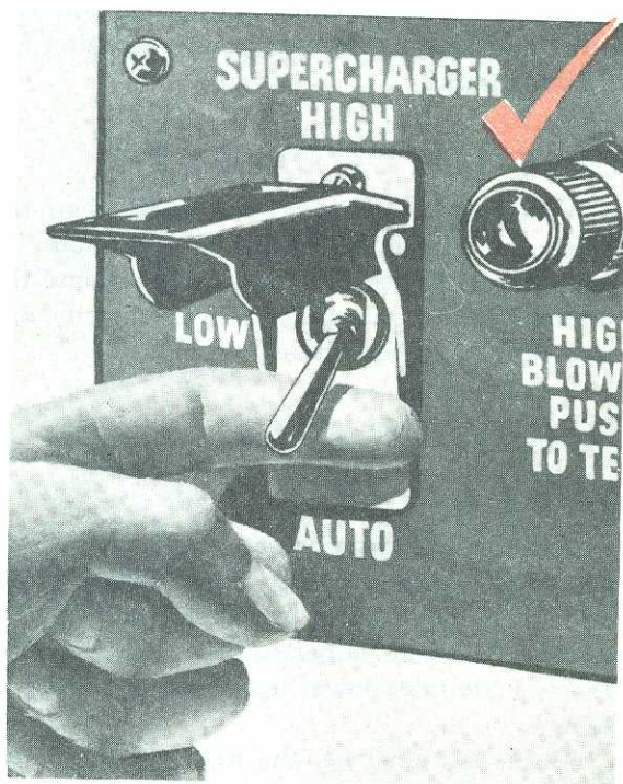
TESTING HIGH BLOWER ON THE GROUND
